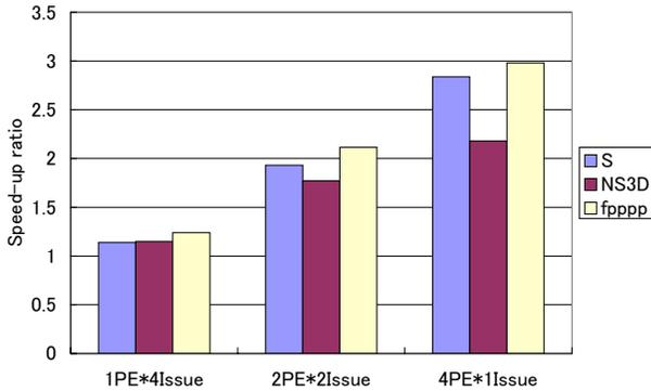
Figure 2: Multiple issues processor cores vs. single issue processor core SCM
