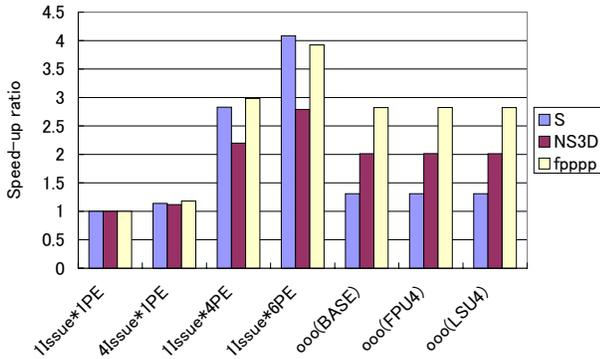
Figure 3: Simple processor core SCM vs. out-of-order processors
