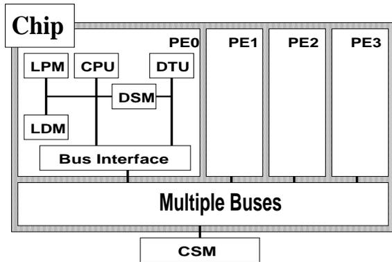
Figure 1: OSCAR type architecture.
